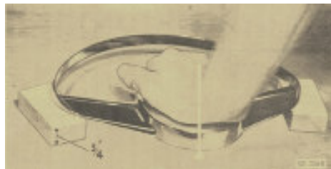
Imparting a slight bend set to Horn Ring
