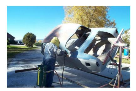
There are many ways attempted to remove rust from an old car, wire brush, chemical stripping, grinder-sander, and many other methods best not mentioned. But, the only way that really works for the average restorer is "media-blasting." All the other methods are a waste of time and many parts are ruined by their use.
